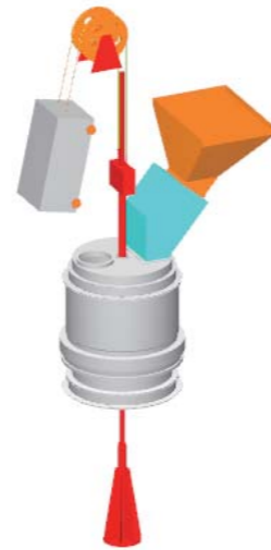
旋转布料系统三维设计图 Three dimensional design diagram of rotary distribution system
