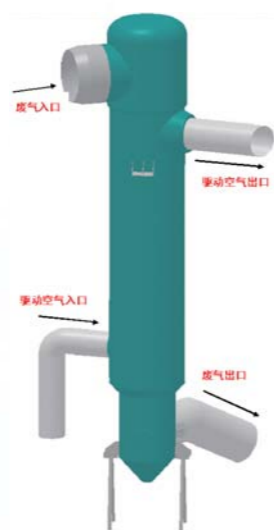
换热器三维设计图 Three dimensional design diagram of heat exchanger
